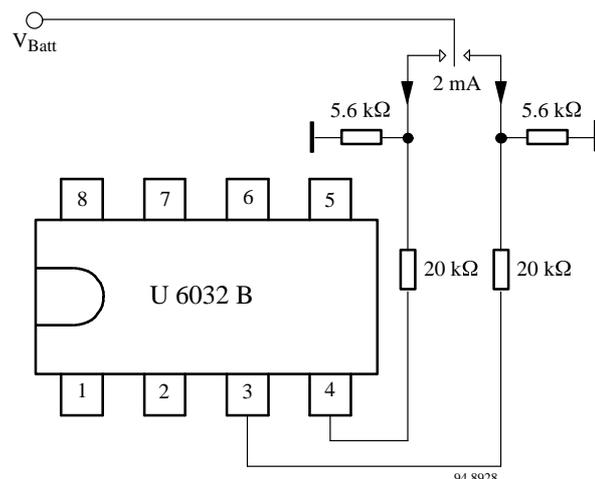
Figure 6 Increasing the contact current by parallel resistors
