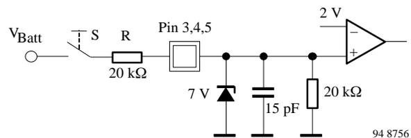
Figure 5 Input circuit
