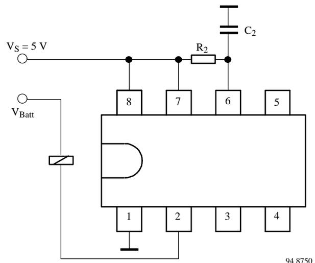
Figure 2b Basic circuit for  $V_S = 5 \text{ V}$
