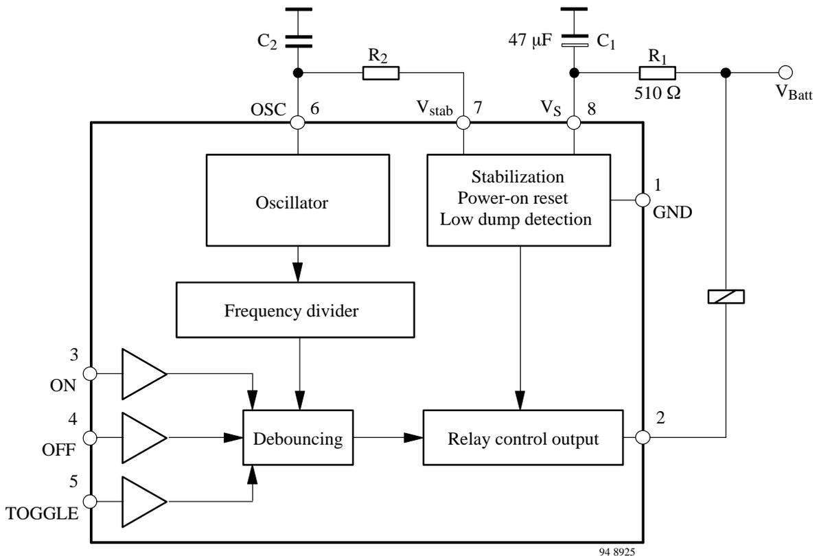
Figure 1 Block diagram with external circuit
